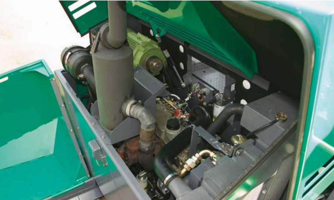
The SUPER 1800-2 is powered by a modern, liquid-cooled PERKINS engine rated at 129.6kW. The speed ranges MIN, ECO and MAX are available which select conveniently at the push of a button. ECO Mode is sufficient for 70 to 80% of all paving jobs. This mode reduces fuel consumption, wear and noise emissions.
