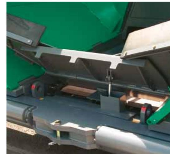
Like all VÖGELE pavers, supply of the SUPER 1800-2 with mix is a clean and safe process passing off swiftly. Thanks to a hydraulically operated hopper front (option), the mix inside the material hopper is directed right onto the conveyors and the entirety of mix properly conveyed in front of the screed.
